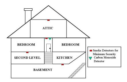
**CARBON MONOXIDE DETECTION:** Detection is required in all sleeping areas of the home. Detection is also required if the home as a fuel burning furnace or boiler and/or an attached garage. Information can be obtained from the Cranford Bureau of Fire Prevention – (908) 709-7360.
