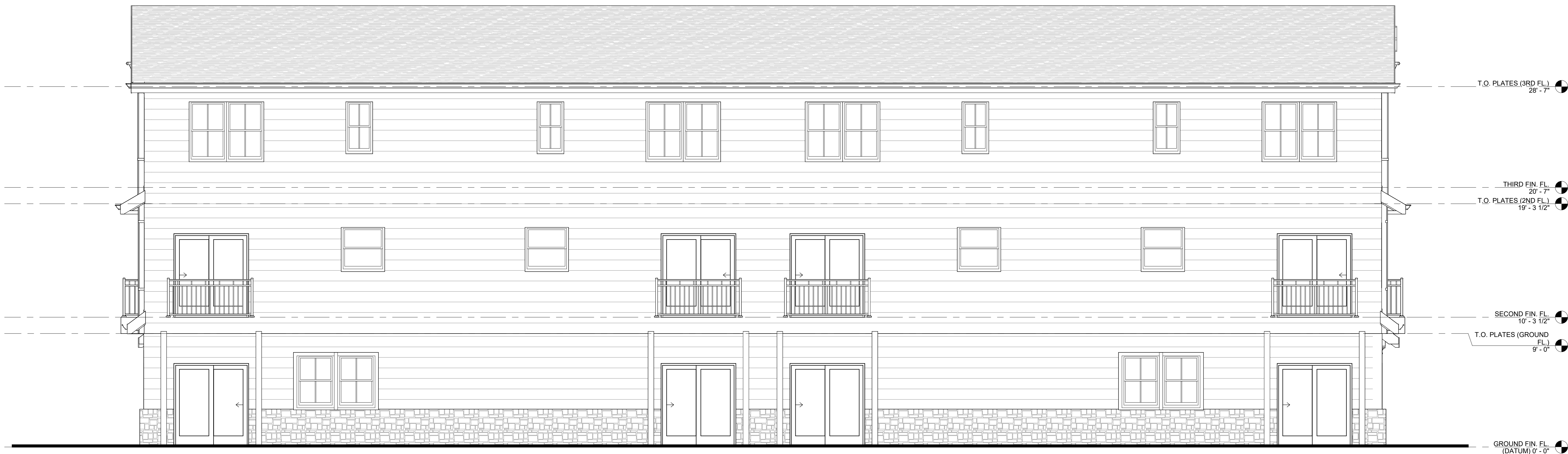
2 BUILDING 1 - REAR ELEVATION SCALE: 1/4" = 1'-0"
