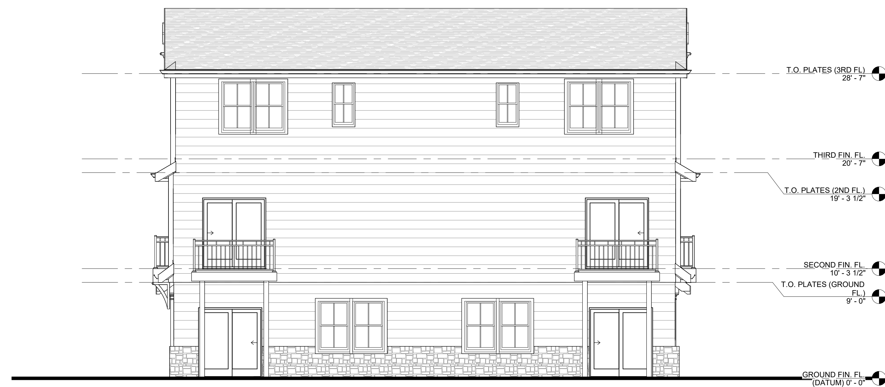
3 REAR ELEVATION (BUILDING-3) SCALE: 3/16" = 1'-0"
