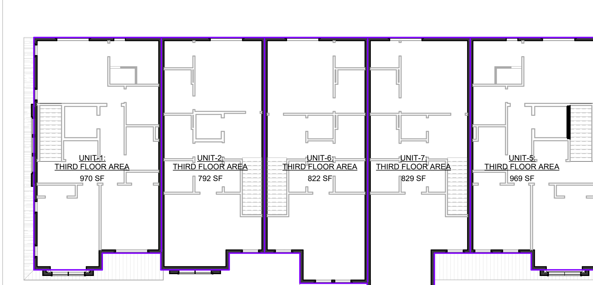
2.3 BUILDING-2 - THIRD FLOOR AREA PLAN SCALE: 3/32" = 1'-0"
