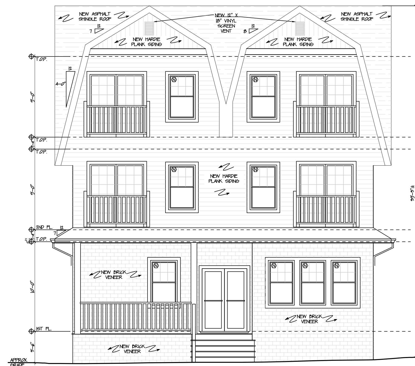
EXIST FRONT ELEVATION W/ADDITION/ALTERATION SCALE: 3/16" = 1'-0"
