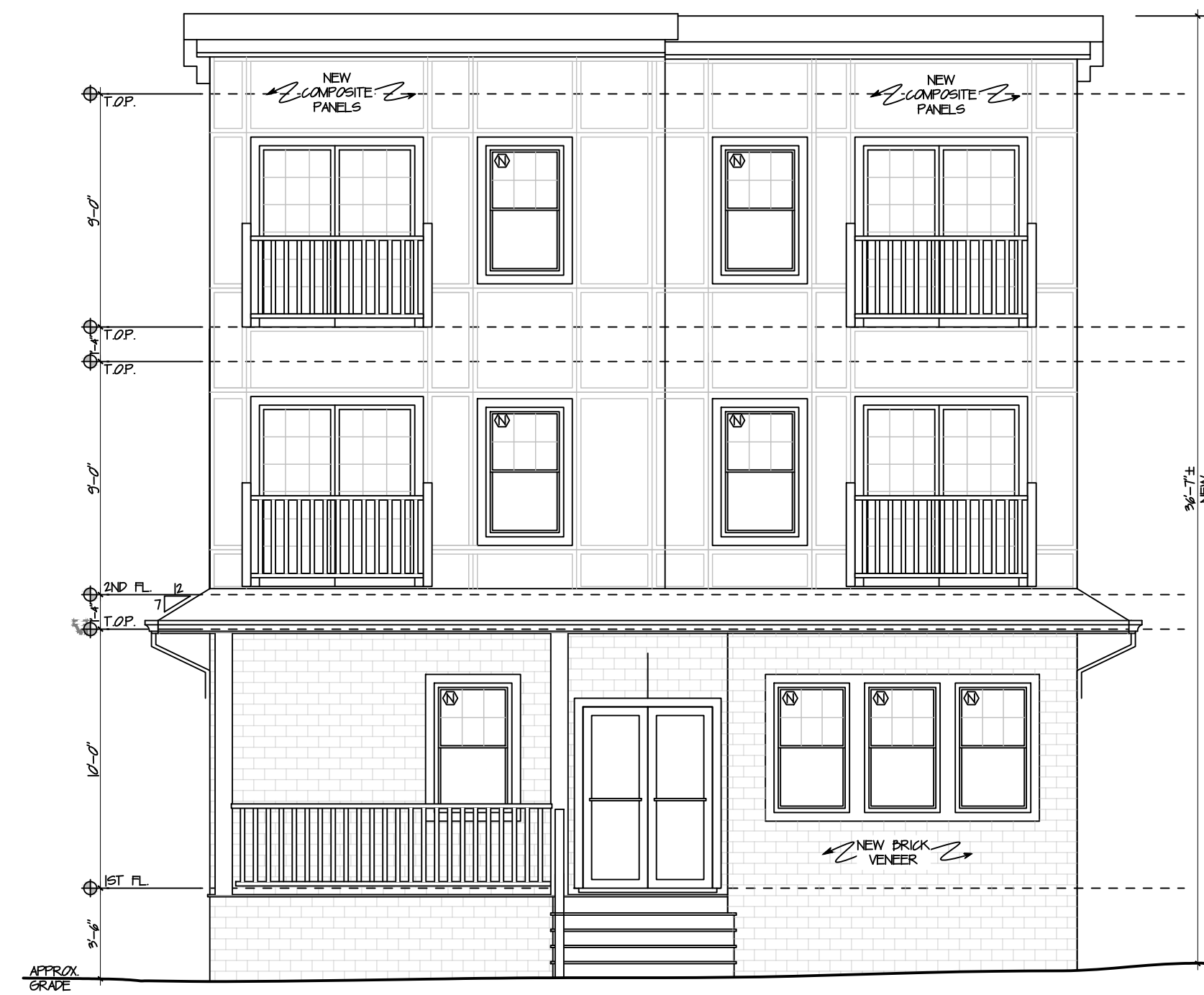
EXIST FRONT ELEVATION W/ADDITION/ALTERATION SCALE: 3/16" = 1'-0"
