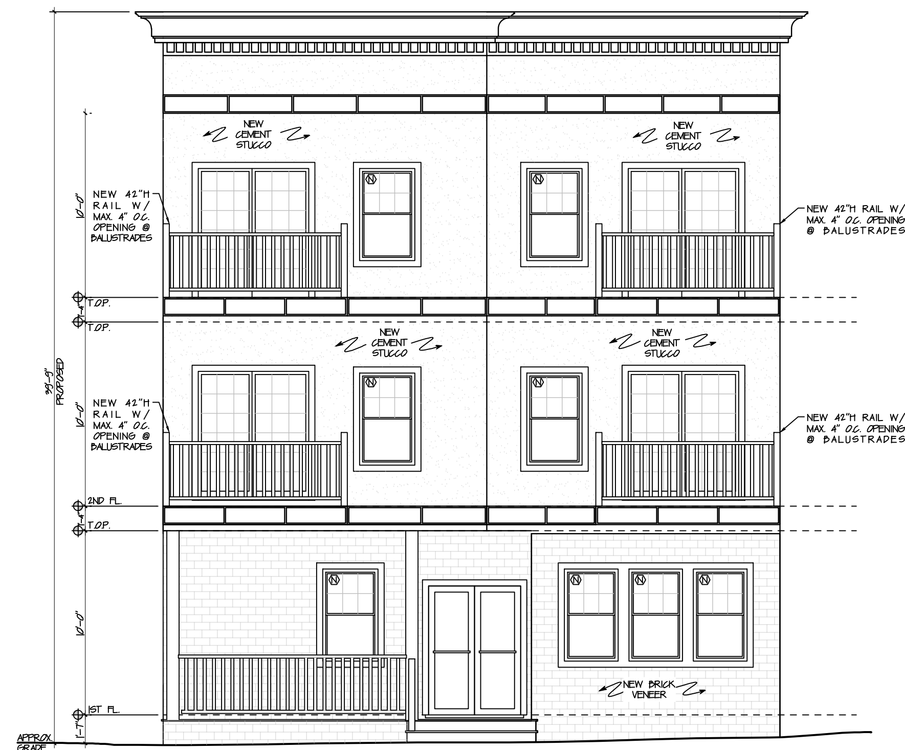
PROPOSED FRONT ELEVATION SCALE: 3/16" = 1'-0"
