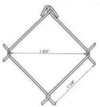
Important: The maximum mesh size for a pool fence is smaller than the standard chain link mesh
