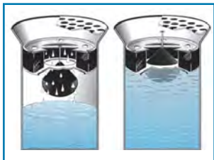
Floor drain float plug.
