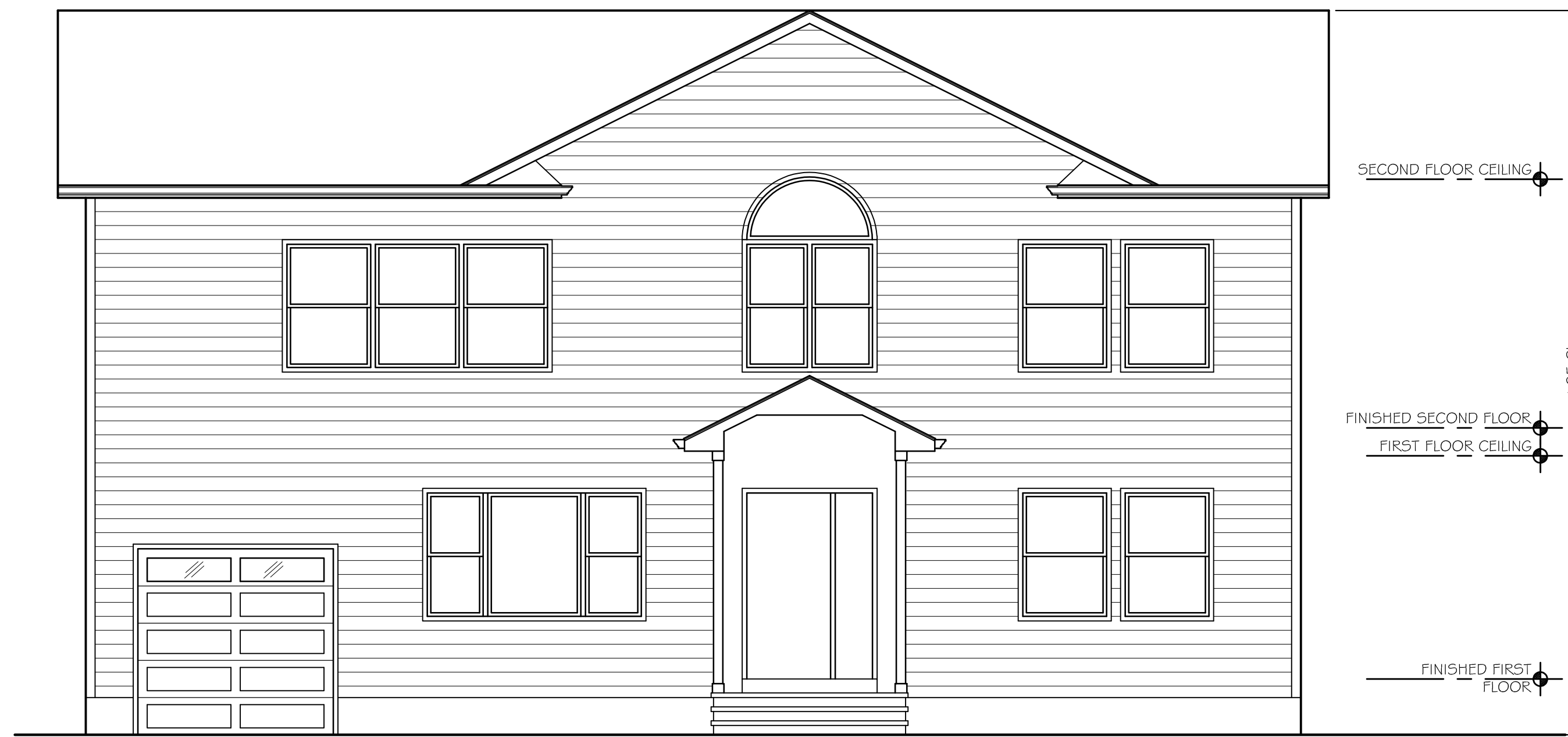
3 V-2 EXISTING FRONT ELEVATION SCALE: 1/4" = 1'-0"
