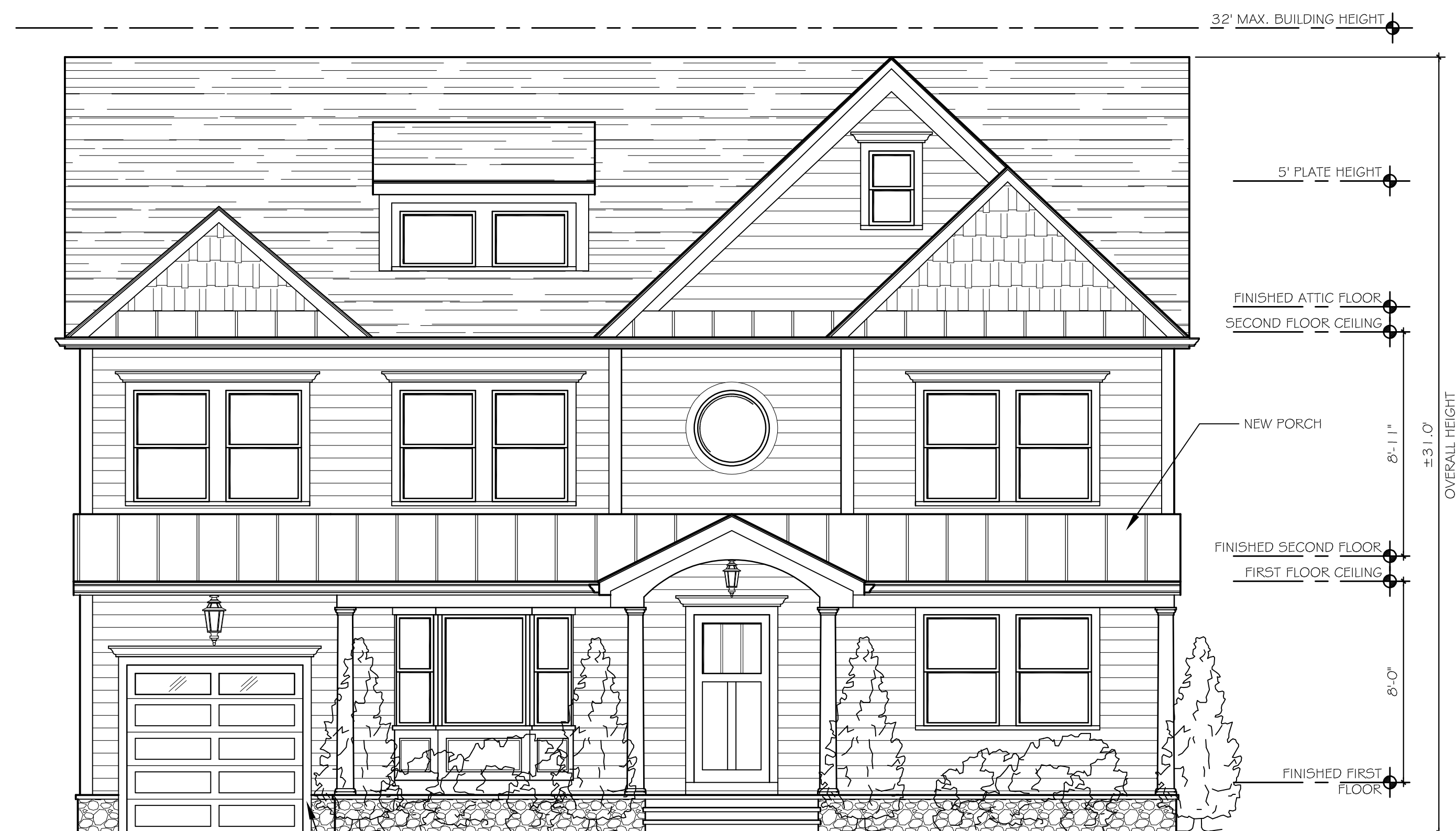
1 V-4 PROPOSED FRONT ELEVATION SCALE: 1/4" = 1'-0"
