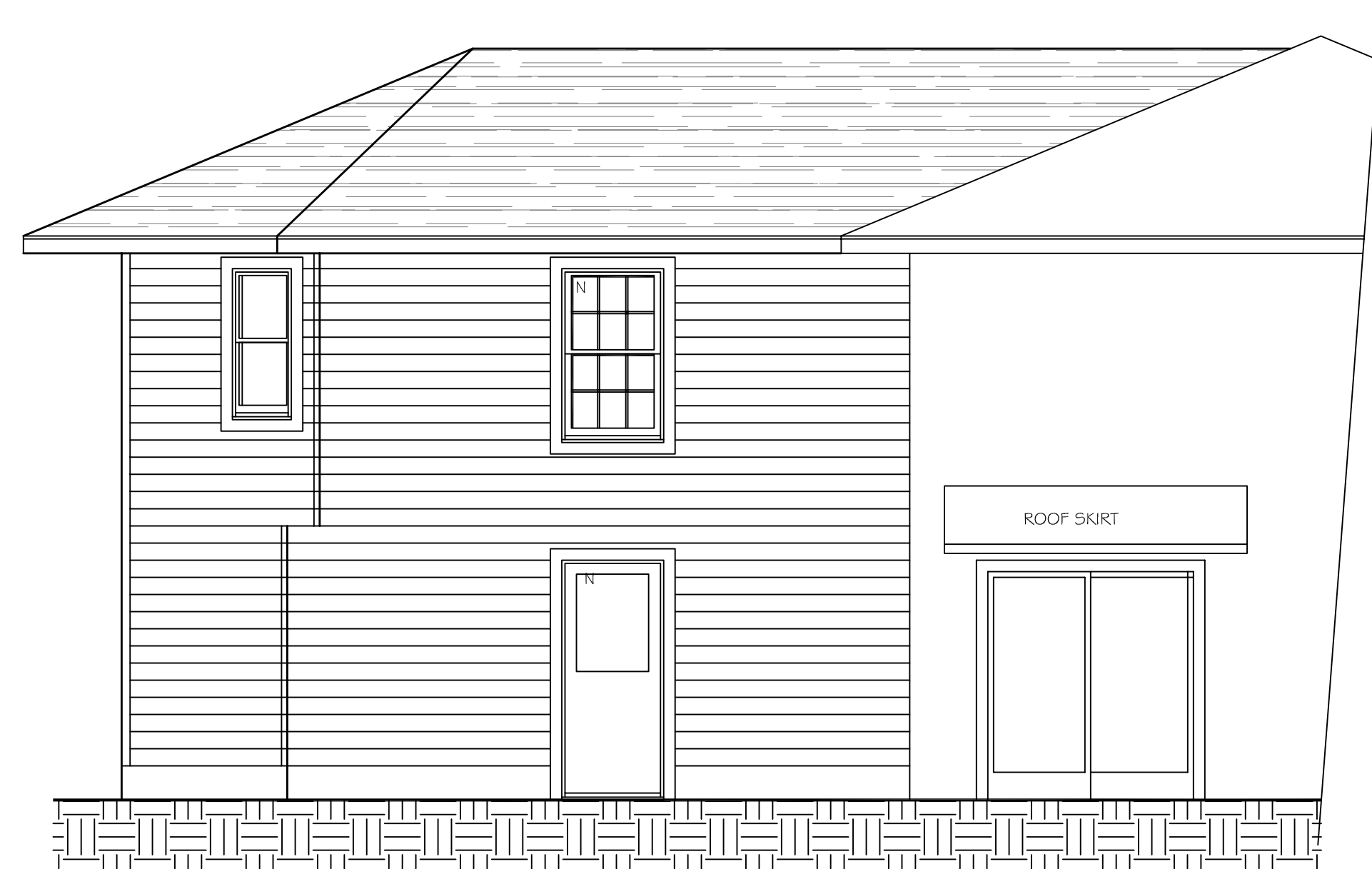
1 A-1 PRELIMINARY REAR ELEVATION SCALE: 1/4" = 1'-0"
