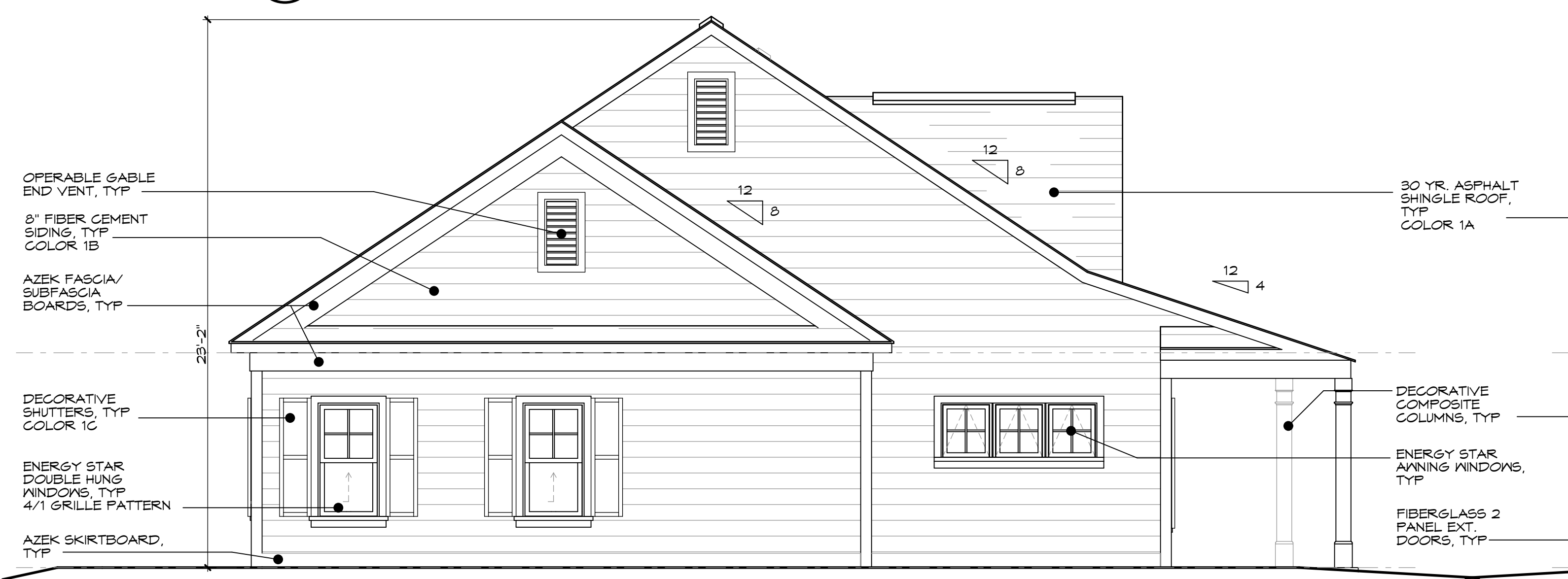
2 BLOCK 573 - LOT 10 PROPOSED LEFT ELEVATION SCALE: 1/4" = 1'-0"
