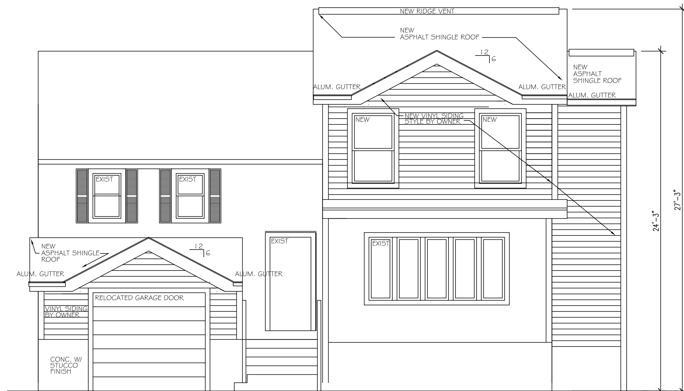
PROPOSED FRONT ELEVATION SCALE 1/4" = 1'0"
