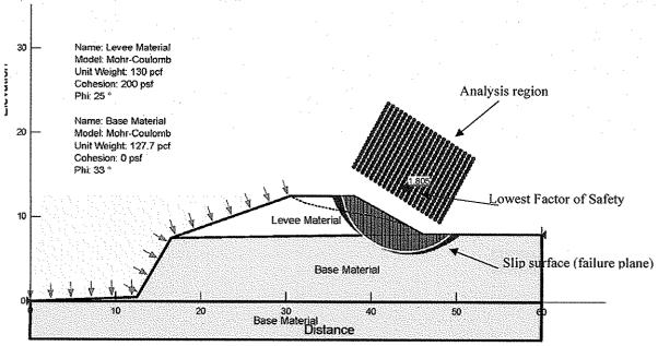
This figure shows the two materials, the water level and the slip circle with the lowest factor of safety. The grid of red dots shows the region where the potential failure circles were centered. The lowest factor of safety is shown as a brighter red dot with the value beside it.
