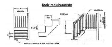
11. Handrails: All stairways with four or more risers require continuous handrails. Handrails shall not be less than 30" or greater than 38" measured vertically from the stair nosing. Handrails shall be continuous the full length of the stairs. Handrails shall be returned or shall terminate to a wall or post. Grip sizes shall be in accordance with the 2015 International Residential Code, New Jersey Edition, Section R311.7.8.3. Type I or II.
