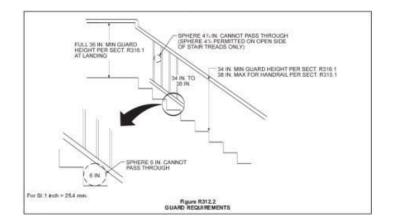
10. Stairways: Minimum stairway width is 36", maximum riser height is 8 ¼", minimum tread is 9". A nosing not less than ¾" but not more than 1 ¼" shall be provided when solid riser are used. Stairways more than 12' above floor level or grade required a landing.
